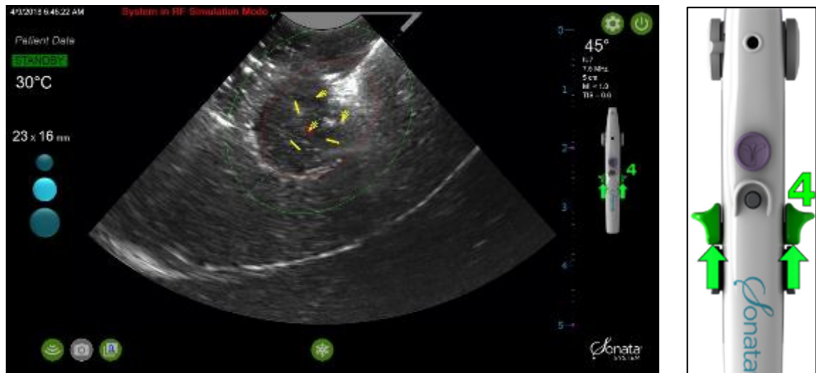
Figure 4-23. Deploy Needle Electrodes by advancing Needle Electrode Sliders forward.
