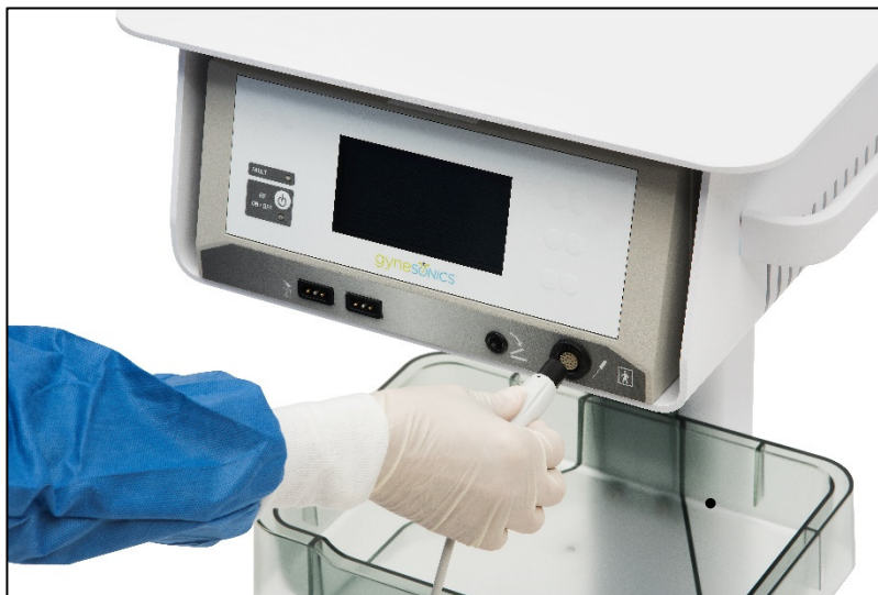
Figure 3-19. Connect RFA Handpiece Cable to front of RF Generator.
