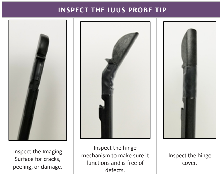
Figure 3-14. Inspect the IUUS Probe Tip before using.
