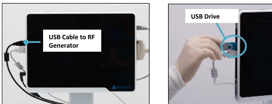
Figure 6-13. Remove USB cable from USB port and insert USB Drive in the USB port.
