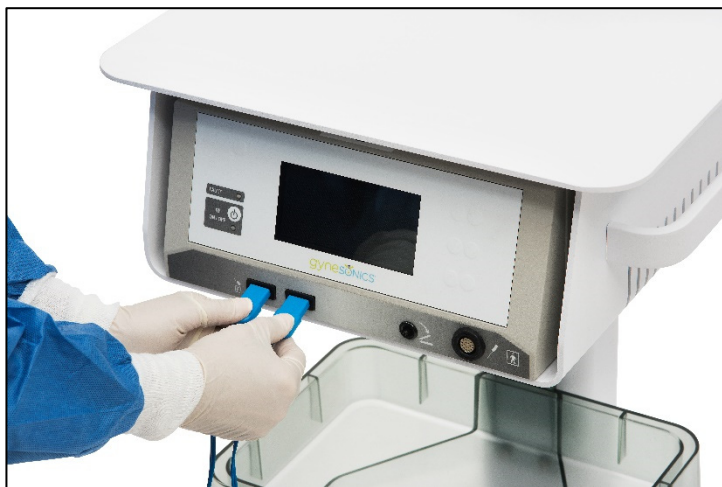
Figure 5-1. Disconnect Dispersive Electrodes Cables from RF Generator.
