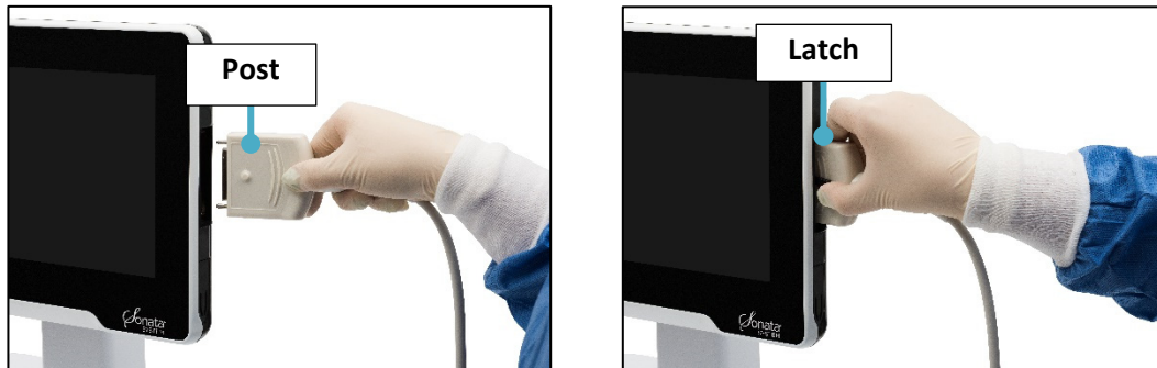
Figure 3-18. Connect IUUS Probe to SMART Tablet and slide latch to lock.
